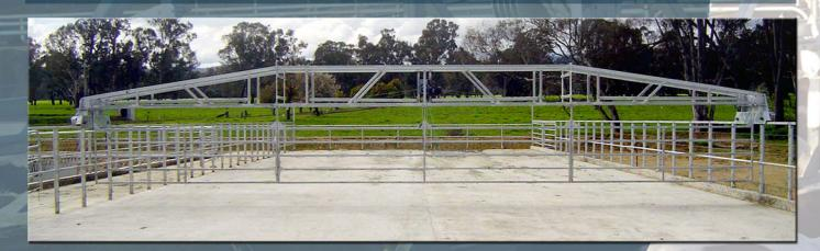
Larsen Dairies Backing Gates are a fully electric operated herd control system. The design provides operators full flexibility over their herd management practices in providing the ability to split large herds. The gate moves back and forth along the yard herding cows toward the dairy saving both time and manpower.
